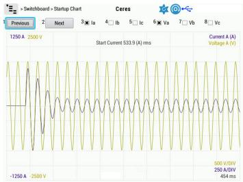
The startup chart displayed on the controller of the Instruct FS unit showing the amperage stabilizing over time. The detail that the startup chart provides enhances the troubleshooting capabilities of the unit.
