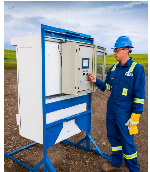
KUDU PCP Manager well optimization unit mounted on a variable frequency drive (VFD).
