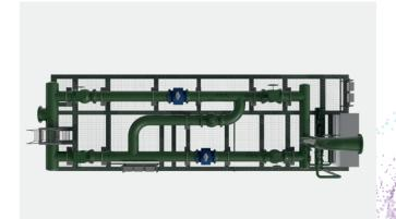
The shows a duty/check configuration where the duty and check meters are routed in series via a cross over, otherwise referred to as a Z configuration, for comparison
