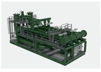
The shows a traditional ultrasonic metering system with a bi-directional prover is shown above. In the image above the prover occupies a second deck below the metering runs adding considerably to the size, weight and complexity of the system. In the event that SVM is deployed without the need for an in-situ prover the complexity, size, weight, pressure drop, CAPEX and OPEX is significantly reduced.
