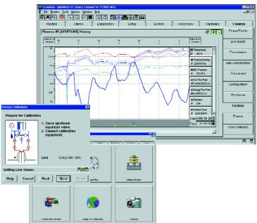
ScanWin Lite Windows interface is used to configure, maintain and manually retrieve data from the Scanner.
