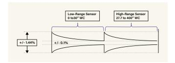
The Sensia Scanner 3100 flow computer offers triple sensorstacking capabilities to support further reduced uncertainties or higher turndown capabilities.
