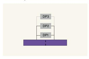
As in the original example, the full-scale value is 400-in WC; therefore, the high-range sensor would be used to measure between 27.7- and 400-in WC. A second DP sensor with a full-scale range of 30-in WC would measure between 2- and 30-in WC. This second sensor could be a Scanner 2000 flow computer communicating serially to the Scanner 3100 flow computer, or it could be a traditional DP transmitter with an analog output.
