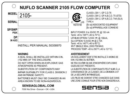
Figure 1.2 - Device serial tag
