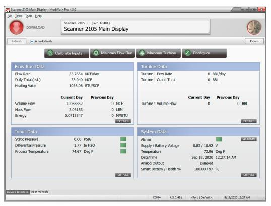
Figure 4.1 - ModWorX software interface
