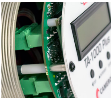
Figure 5.12—Alignment of top circuit assembly over standoffs
