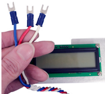
Figure E.11—Switch wires showing two-prong connectors
