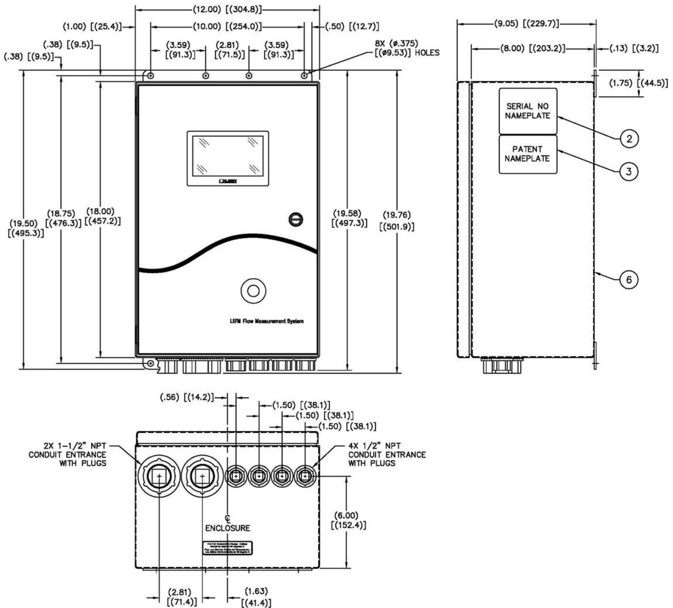
**Figure 2-1: Transmitter Enclosure (units in inches, [mm])**
