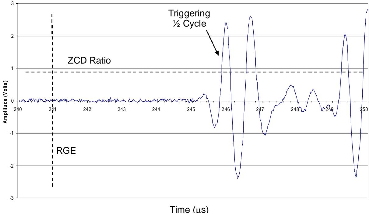
**Figure 6-1: Example Transducer Waveform**
