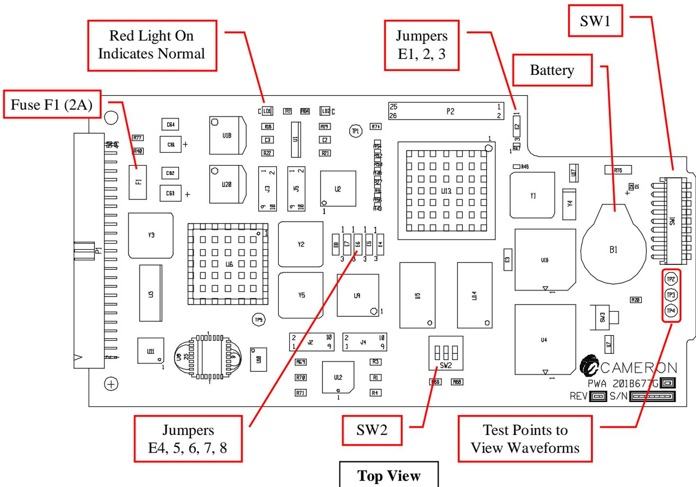
**Figure 5-2: CTC Fuse, Switch, and Jumper Locations**
