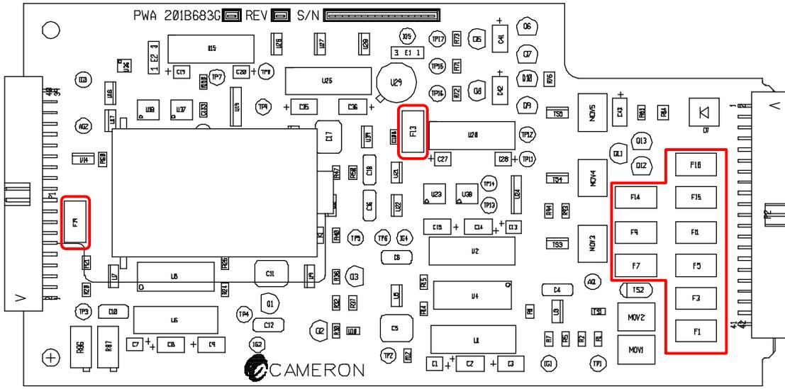
Figure 5-4A: IOB Fuse Location – Top View
