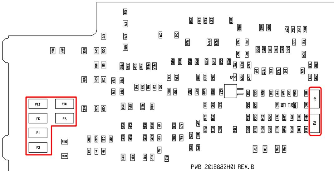
Figure 5-4B: IOB Fuse Location – Rear View
