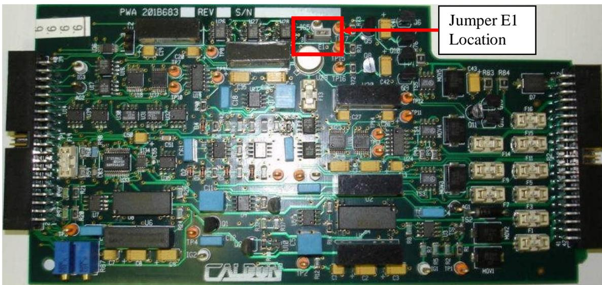
Figure 5-6: Jumper Location to change Digital Output Voltage
