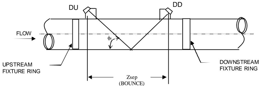
**Figure 3-1: External Diagonal Transducer Bounce Path**
