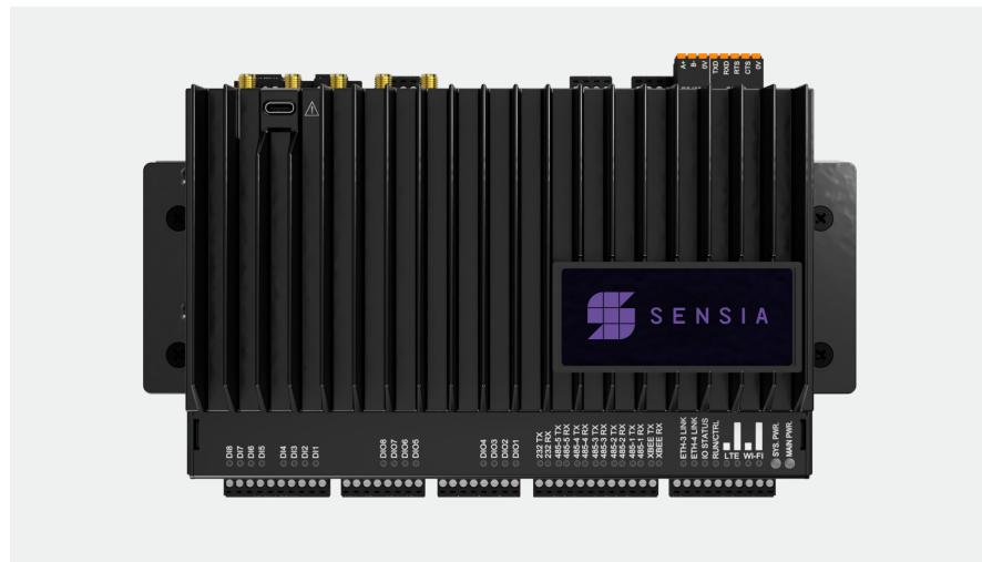
**Combining an edge computer, real-time processor, industrial I/O, GPS, cellular modem, Wi-Fi, and an Ethernet switch into one rugged platform, the QRATE HCC2 edge controller provides analysis and autonomous control for remote equipment.**
