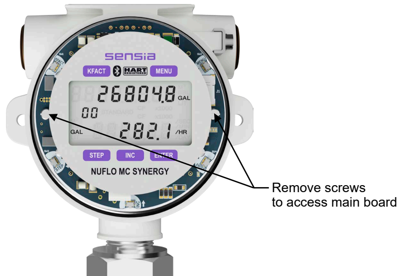
Figure A.10—Removal of faceplate assembly
