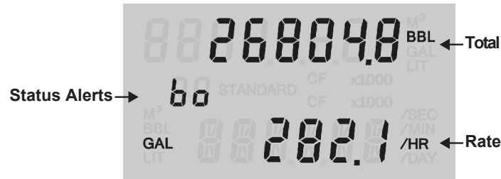
Figure 1.4—Total and Rate are displayed by default. Selected units of measurement are displayed to the right of the total and rate values.
