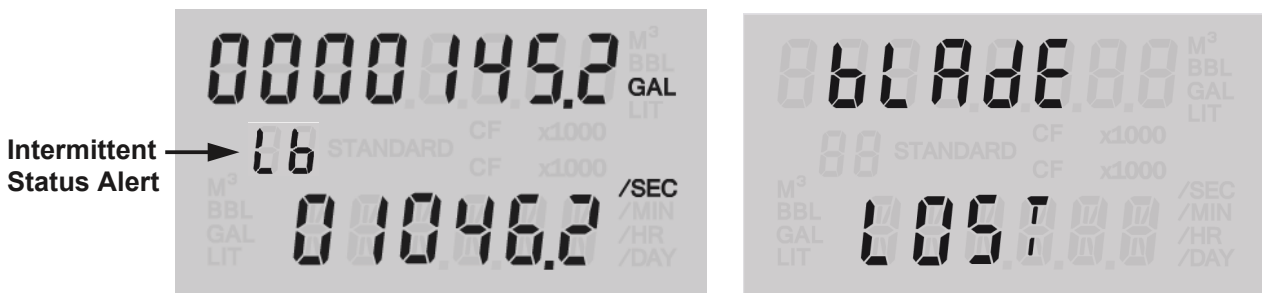
Figure 1.9—A turbine health alarm message (right) is preceded by a momentary two-digit status alert upon detection of a meter health vulnerability such as a missing or lost blade.
