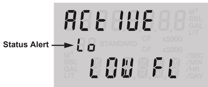
Figure 1.8—Turbine flow alarm display
