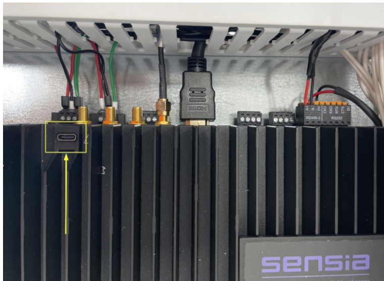
Figure 5.1—HCC2 USB-C connector for laptop connection
