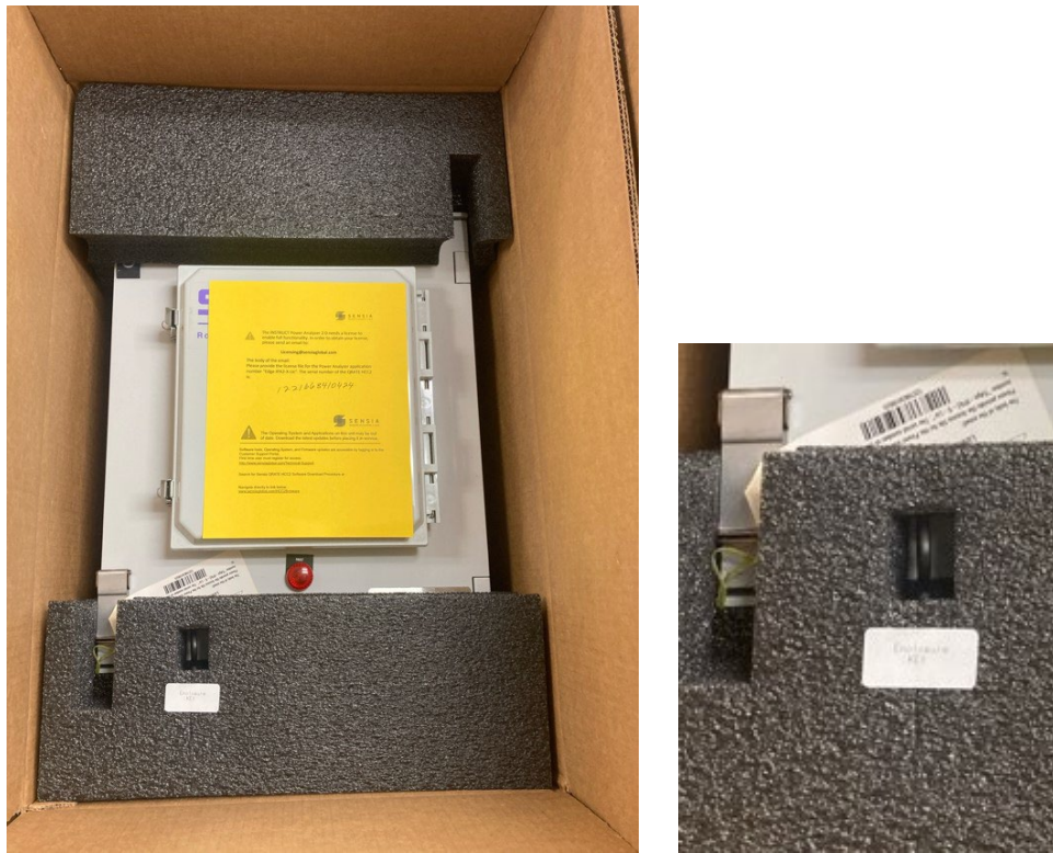
Figure 4.3—Instructions on yellow card (left) and latch key secured in shipping foam (right)
