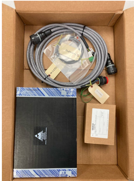
Figure 4.2—PowerDAQ, sensors, and connecting cables
