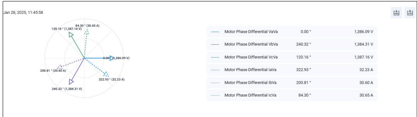
Figure 8.3—Avalon phasor diagram
