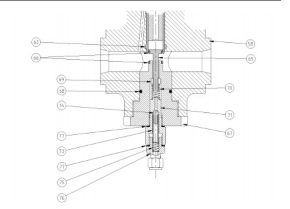
The Bottom Plug Assembly is unscrewed from the Cell Sampler Body using the 'C' Spanner provided in the Special Tool Kit. Note the location of any shims located between the Bottom Plug and the Cell Sampler Body. These will be retained on the Bottom Plug by 'O' Ring (68).
