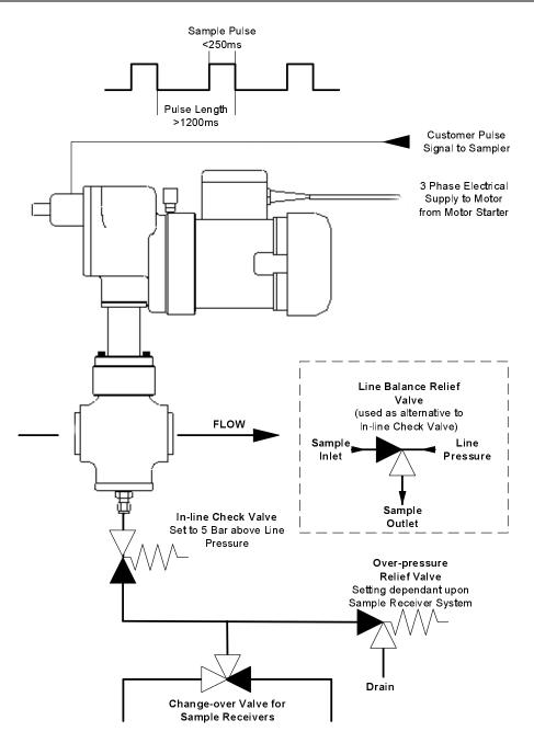
The Check Valve will normally be set to 5 Bar above the maximum line pressure, ensuring that this is sufficient to allow for any additional pressure increase created by thermal expansion when any isolating valves are closed and the effects of trace heating and or solar energy. If the cracking pressure is set too low, the valve may open under adverse conditions, causing the Sample Receiver System to overfill and the sample to leak through the relief valve to atmosphere.
