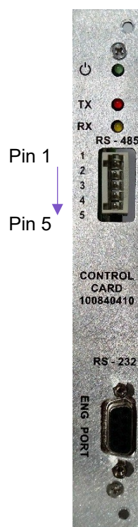
Figure 4-1: INSTRUCT Control Card RS-485 Port
