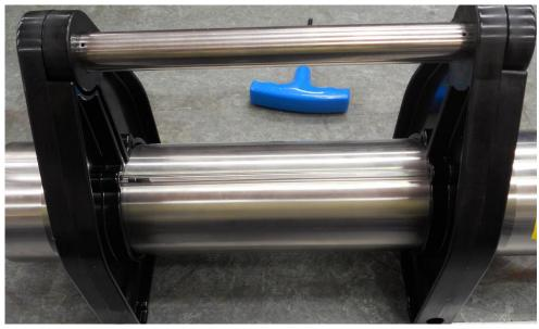
Stand the CPC on its feet and fully tighten the clamping screws whilst keeping the feet flat on the workbench.
