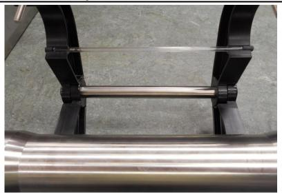
Remove any remnants of the old Level Indicator from the locating grooves in the Mounting Clamps.
