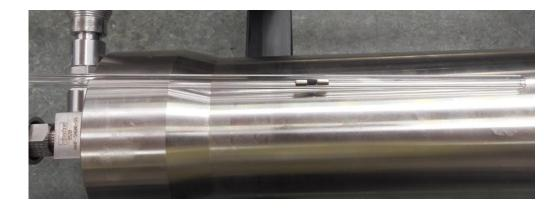
If the magnets are correctly aligned they will stay in position while the tube moves.
