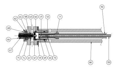
Before removing the Sample Head Assembly, take particular note of the position of the Head in relation to the Support Tube and the gap between the Stop Ring and Sample Head.
