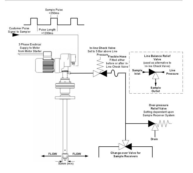
The Sampler will be supplied with the Motor facing across the pipeline, but may be rotated through  $90^{\circ}$  by removing the 4 off M5 Cap Head Screws (48) and turning the Mounting Tube/Gearbox Assembly. Under no circumstances must the Lock Nut (44) be loosened and the Mounting Tube rotated in the Gearbox Housing as this will disturb a critical internal alignment.
