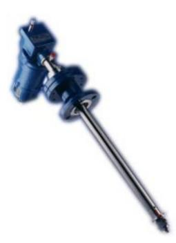
The 710 Electric Sample Probe provides a means of extracting a sample from liquids flowing in a pipeline. Designed for applications where instrument air is unavailable, the 710 Probe is installed directly into the main pipeline.
