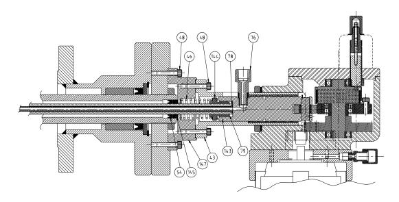
Remove the 4 off M5 Cap Head Screws (48) retaining the Mounting Tube (43) to the Adapter Block (147), noting the orientation of the Motor/Gearbox Assembly to the Support Tube Flange.
