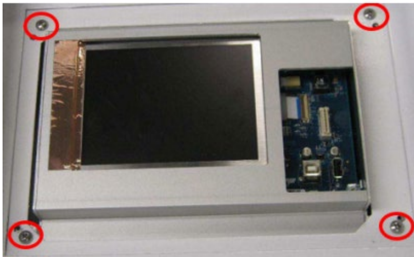
Figure 8-3 - Controller Bezel Removed
