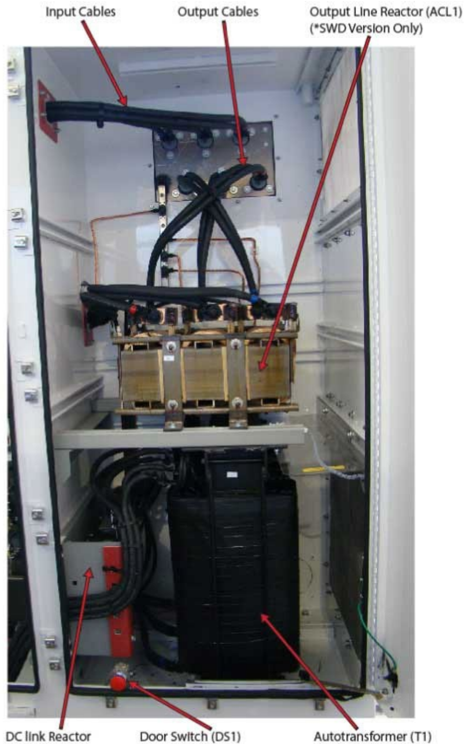
Figure 1-3: Sensia ES7, 18P Series Transformer Compartment (interior of 454 kVA shown)
