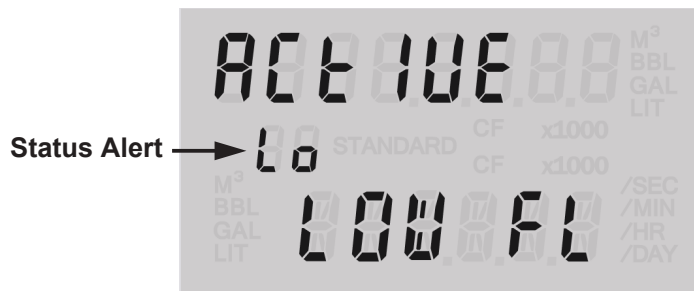
Figure 1.7—Turbine flow alarm display
