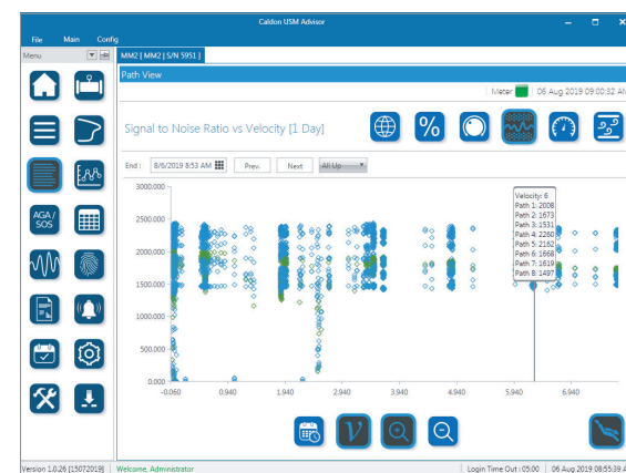
Historical signal-to-noise ratio vs. velocity trend at Path View
