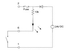
Figure 7 - Connecting a Digital Input<sup>1</sup>
