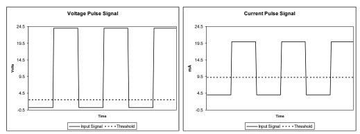
Figure 9 - Voltage and Current Pulse Signals<sup>2</sup>
