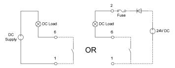
Figure 8 - Connecting a Digital Output<sup>1</sup>
