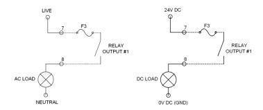
Figure 2 - Connecting a Relay Output
