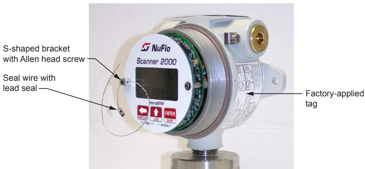
Figure A.20—Measurement Canada seal kit components
