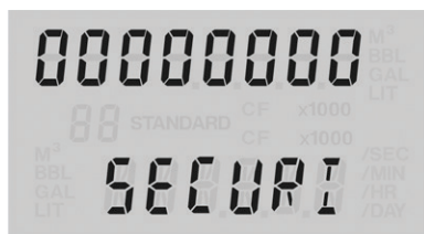
Figure 1.11—LCD display of security password menu
