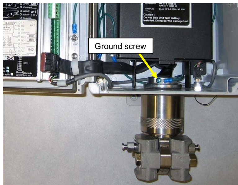
Figure 2.2—Proper positioning of the DPE+ transducer (shown with a Scanner 1140)
