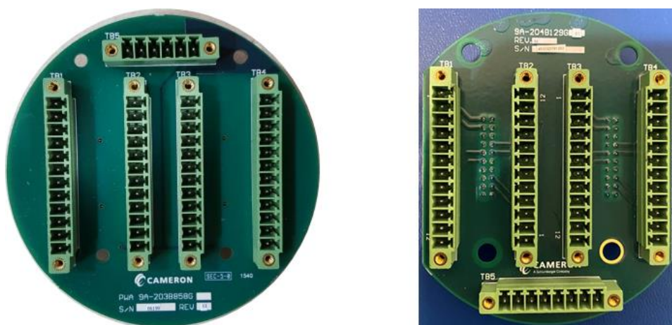
Figure 3.2 Locations of Terminals on Electronics MXR Board for Legacy (left) and NextGen (right) meters
