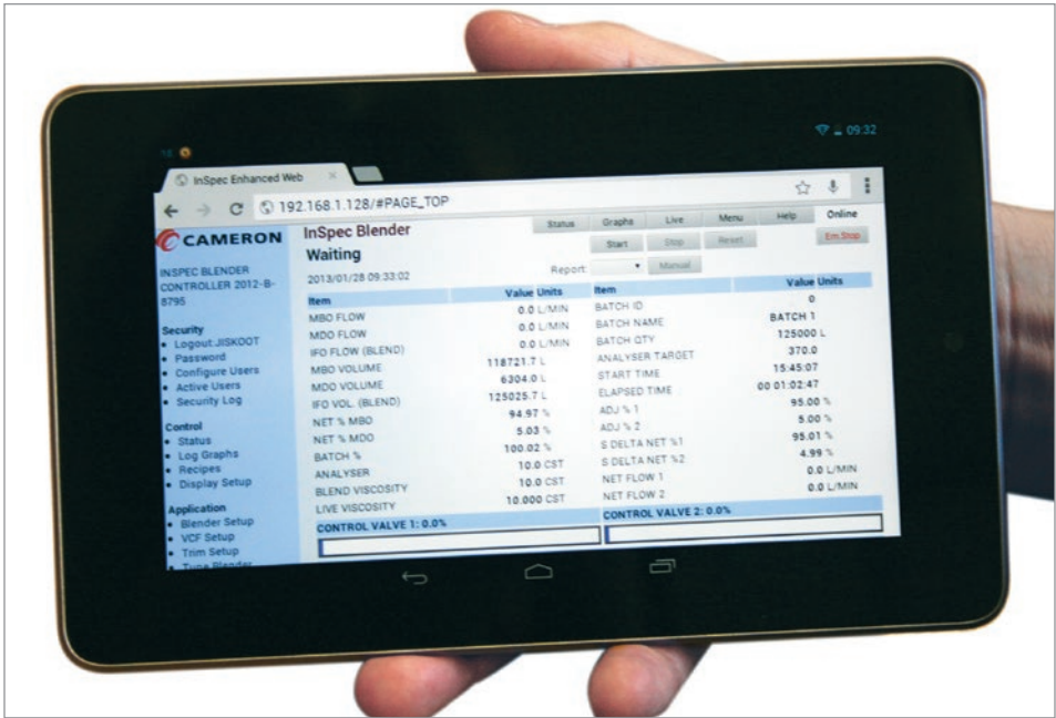
Controlled rate with trim —Controlled rate blender with analyzer feedback to control quality.
