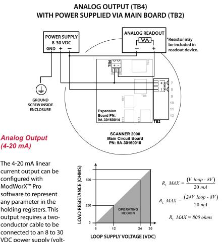
required to power the instrument for a given loop resistance. In addition, the mathematical relationship between loop voltage and load resistance is given. For example, if a power supply voltage of 24 volts is available to power the current loop, the maximum load resistance would be 800 ohms.
