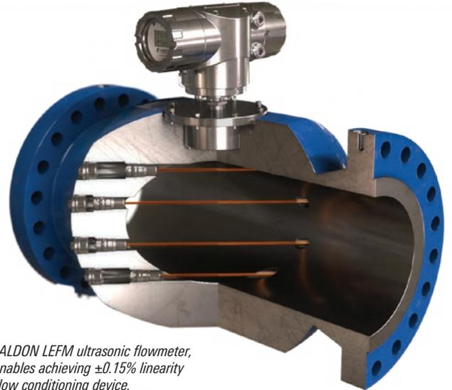
*240Ci CALDON LEFM ultrasonic flowmeter, which enables achieving  $\pm 0.15\%$  linearity with a flow conditioning device.*
