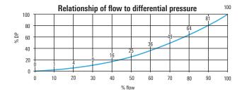
What is usually observed is that turndown is not caused by the limitation of the differential-pressure-producing device but by the ability to precisely sense the differential pressure. DP sensor stacking is a method to reduce uncertainty. In regard to the values presented in the subsequent example, the evaluator should consider possible limits and the additional uncertainty of the specific DP producer.
