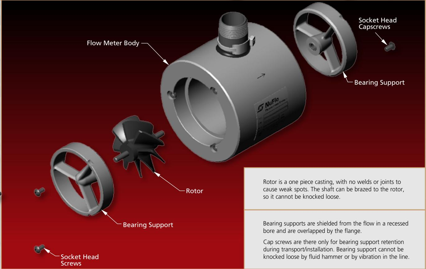
Rotor is a one piece casting, with no welds or joints to cause weak spots. The shaft can be brazed to the rotor, so it cannot be knocked loose.
