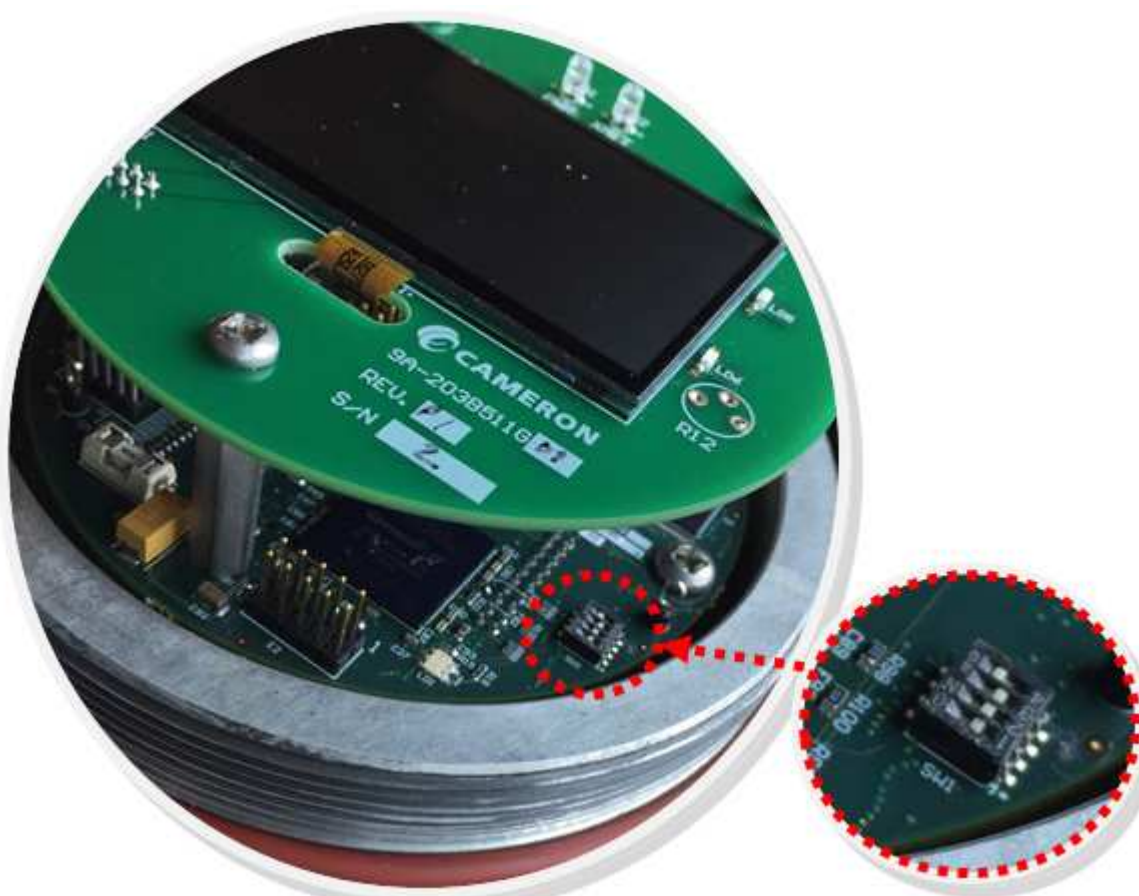
Figure 9-1 Transmitter, Cover Removed - SW1-4 set to prevent configuration changes (shown without tamper evident seal for clarity)
