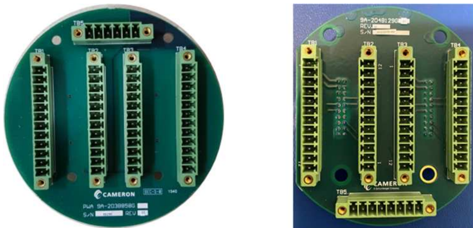
Figure 3-6 - Locations of Terminals on Remote Interface Board for Legacy (left) and NextGen (right) meter bodies.
