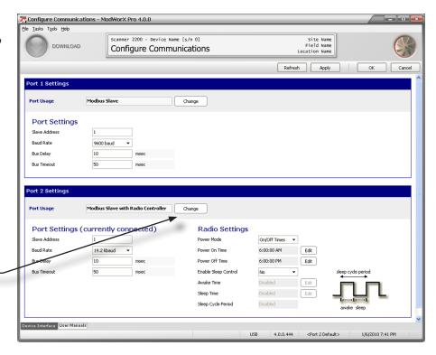
In the Port 2 Settings section, change the Port Usage field to Modbus Slave with Radio Controller.
