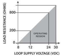
$$R_L \ MAX = \frac{\left(V \ loop - 8V\right)}{20 \ mA}$$
