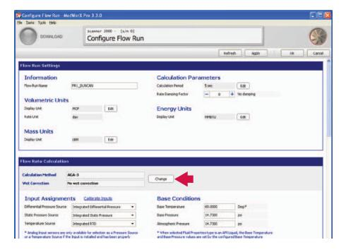
5. From the Change Flow Run Calculation Methods screen, select the Fluid Properties Calculation Method that is appropriate for the type of fluid being measured.
