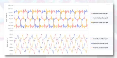
After few operational actions were taken, the harmonics distortion was reduced by 84%, which immediately showed an important effect over the quality of the power delivered to the motor. The change was easily identified visually in the electrical signal waveforms, and the power efficiency indicators generated by the PA 2.0.
