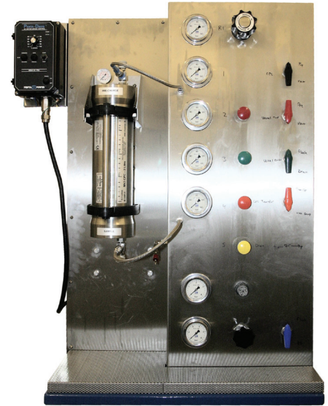
JISKOOT ShearMix constant-pressure-cylinder mixing station.
