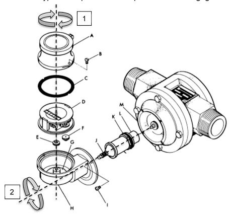
The register position of item (D) can be changed in any combination of two axis (1 or 2) in 90-degree increments.
