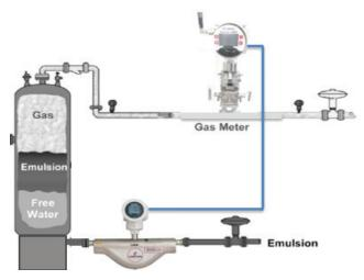
Two-phase separator using a Coriolis flow meter for watercut measurement.
