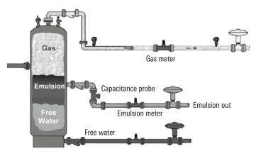
Three-phase separator using a water and oil ratio analyzer (emulsion meter) for water-cut measurement.
